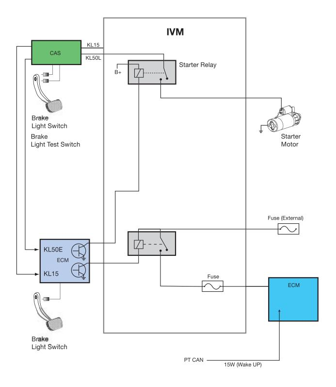
**Actuation Time of Terminal 50:** The monitored actuating times of terminal 50 protects the starter against overloading. The actuation times of terminal 50 are:
